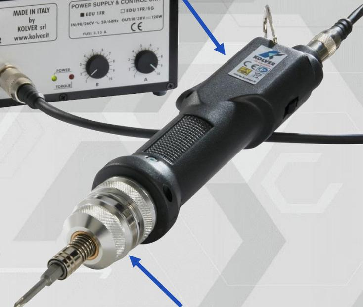
Torque is adjusted at the front of the screwdriver
