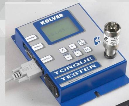
\* torque tester is required to calibrate and check torque
