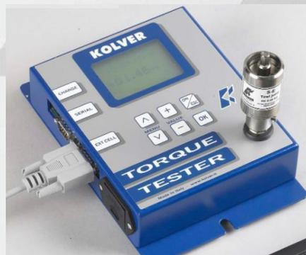
\*A torque tester is required to calibrate and check torque
