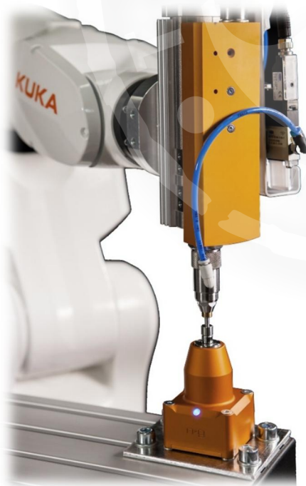
Cyclic torque verification inside the automated assembly system
