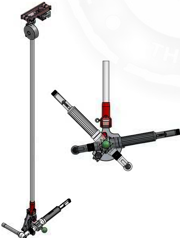
DMFi 200 with swivel and indexable tool clamp
